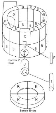
The MIFCO furnaces have been designed so that relining is rapidly and easily done. Complete relining kits are available as a package unit. These kits include all replacement refractory shapes, insulation and the correct type of refractory mortar. Structural parts of the furnace which are subject to normal abuse, and may need replacement, are available. Relining procedure is as follows:
