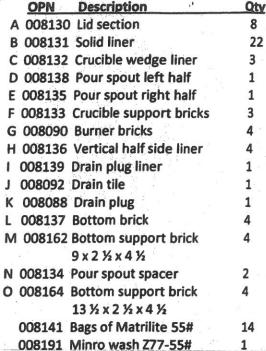
The MIFCO furnaces have been designed so that relining is rapidly and easily done. Complete relining kits are available as a package unit. These kits include all replacement refractory shapes, insulation and the correct type of refractory mortar. Structural parts of the furnace which are subject to normal abuse, and may need replacement, are available. Relining procedure is as follows:
